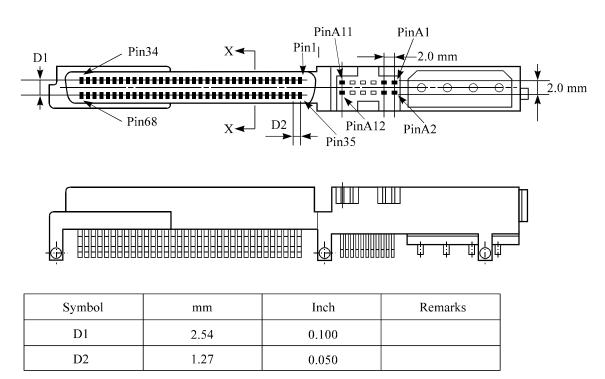
The tolerance is  $\pm 0.127$  mm (0.005 inch) unless otherwise specified
